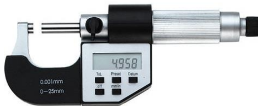
Figure 24: Example of millesimal micrometer for external dimensions
