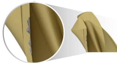
Figure 19: Example of band chipping
