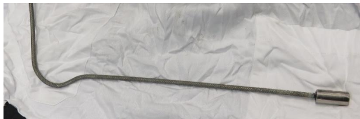
Figure 5: "S"-shaped bend in the cable following failure to apply manual tension to the first 50 cm of cable
