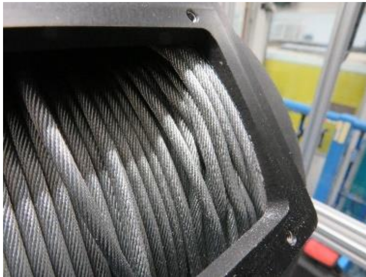
Figure 3: Example of an anarchic winding
