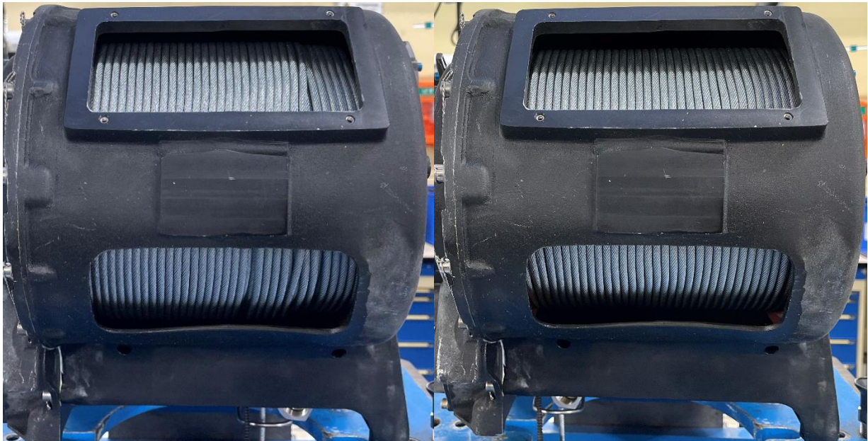
Figure 1 : On the left, example of a winding showing gaps following cable penetration. On the right the same hoist wound with a load to tighten the turns of the lower layers.
