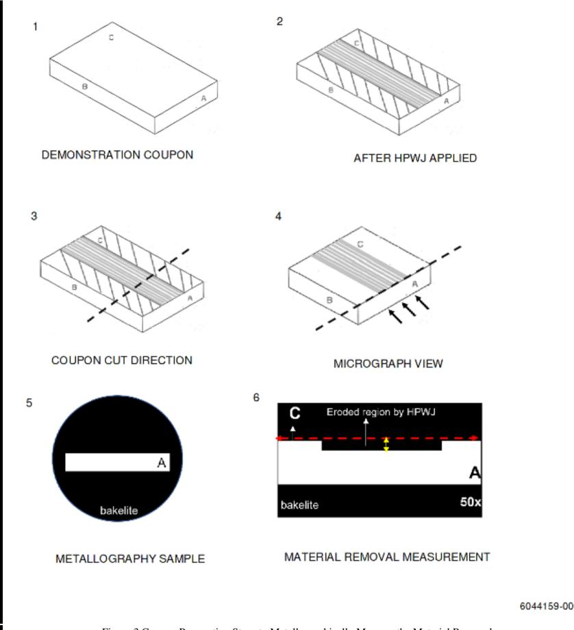
Figure 3 Coupon Preparation Steps to Metallographically Measure the Material Removal
