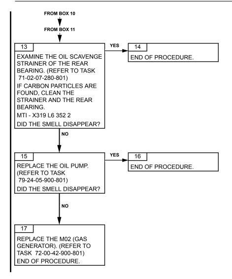
Failures observed during engine operation71-00-06-814-807-A01Page 105Oct. 30/2018
