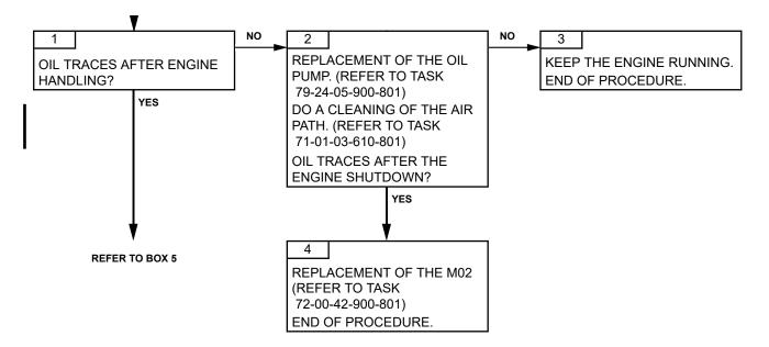
Failures observed during maintenance
