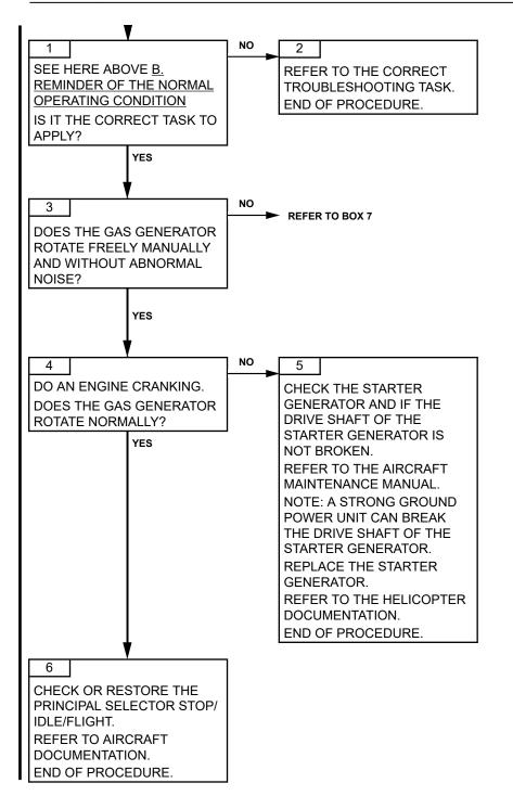
Failures observed during engine operation Page 102 Apr. 15/2020
