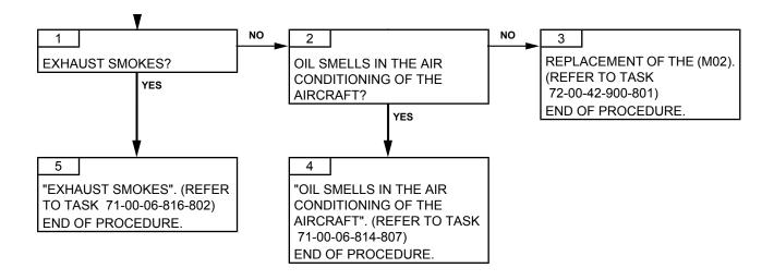
Failures observed during maintenancePage 10271-00-06-816-815-A01Aug. 30/2011
