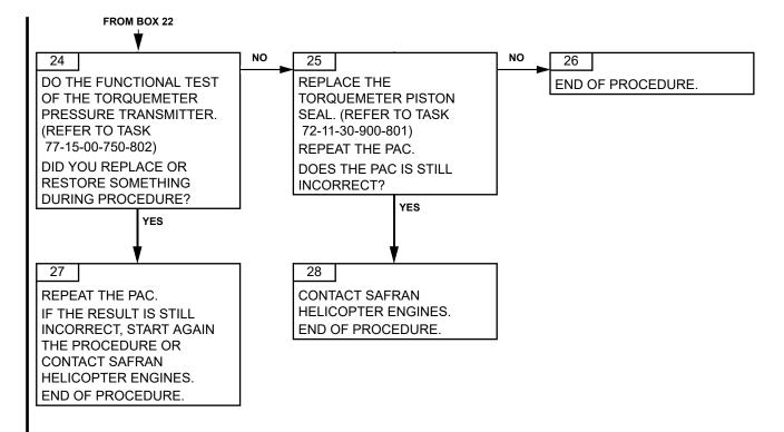
Failures observed during transient rating<br/>Page 10771-00-06-813-810-A01Page 107<br/>Apr. 15/2022
