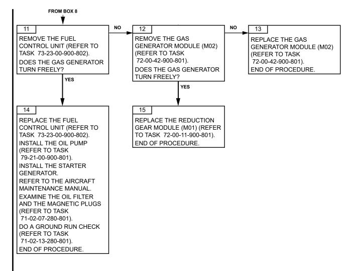
Failures observed during engine operation Page 104 Apr. 15/2020
