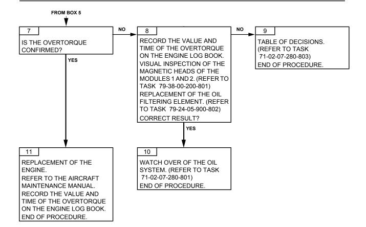
Failures observed during engine operationPage 10371-00-06-814-811-A01Feb. 28/2013
