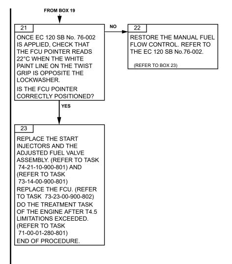
Failures observed during engine operationPage 10671-00-06-812-805-A01Apr. 15/2023
