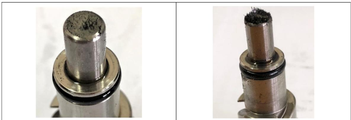
Reference image for the maximum accepted quantity of dust-type particles
