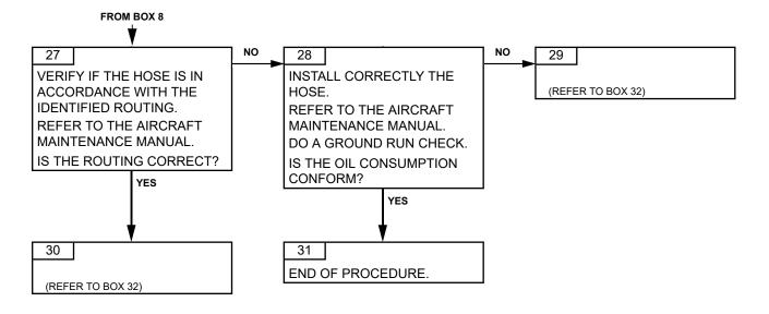
Failures observed during maintenance71-00-06-816-811-A01Page 108Dec. 30/2020
