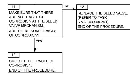
Failures observed during maintenance71-00-06-816-809-A01Page 104June 15/2021
