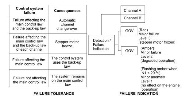
Tolerance and failure indication
