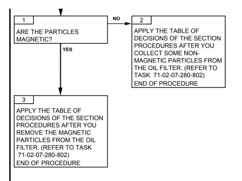
Failures observed during maintenance71-00-06-816-803-A01Page 102May 30/2011
