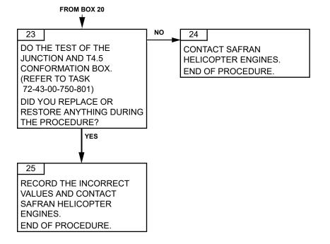
Failures observed during engine operationPage 10871-00-06-812-808-A01Dec. 30/2020
