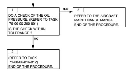
Failures observed during engine operationPage 10271-00-06-814-808-A01Nov. 30/2015
