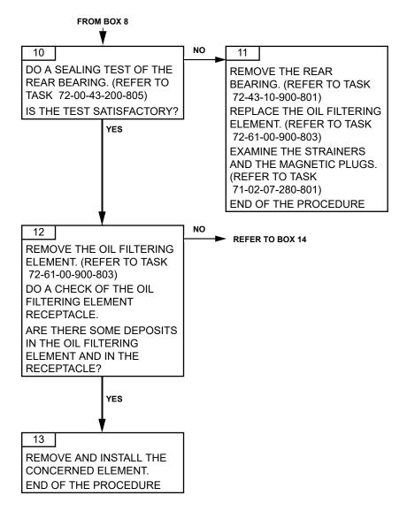
Failures observed during maintenance 71-00-06-816-812-A01 Page 104 Dec. 30/2020
