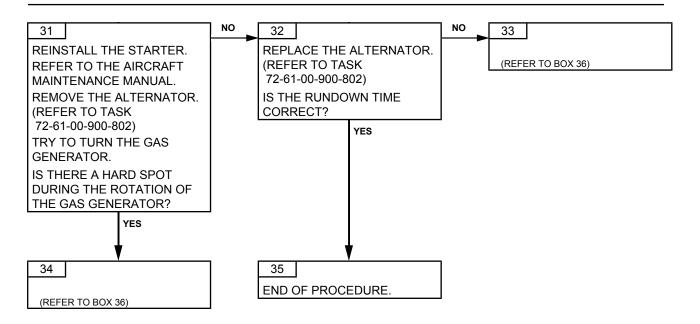
Failures observed during engine operationPage 10871-00-06-815-802-A01Nov. 30/2015
