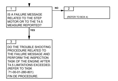
Failures observed during engine operation71-00-06-812-804-A01Page 102Nov. 30/2017Nov. 30/2017
