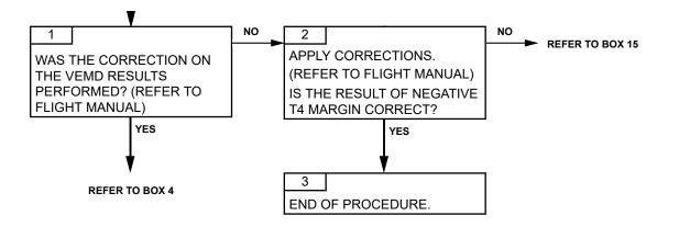
Failures observed during maintenance71-00-06-816-816-A01Page 102June 15/2019June 15/2019
