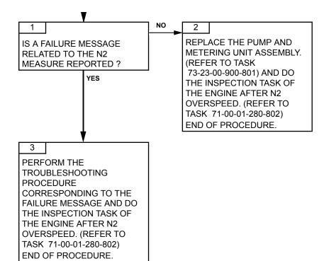
Failures observed during engine operationPage 10271-00-06-814-807-A01Nov. 30/2017
