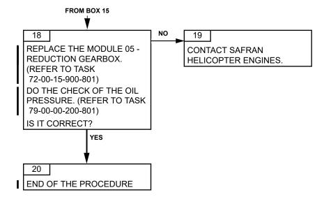
Failures observed during maintenance 71-00-06-816-812-A01
