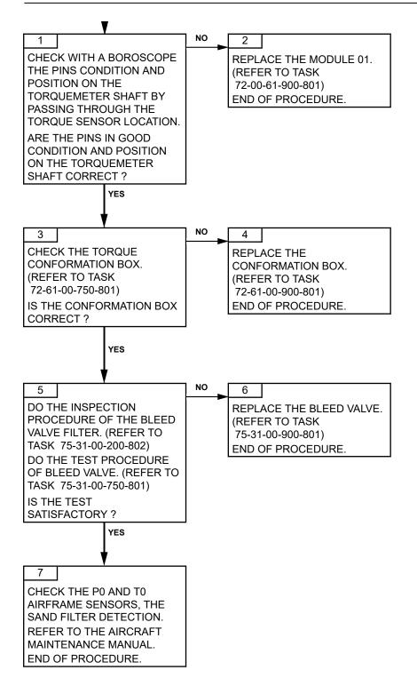
Failures observed during maintenance 71-00-06-816-819-A01 Page 102 Dec. 30/2020
