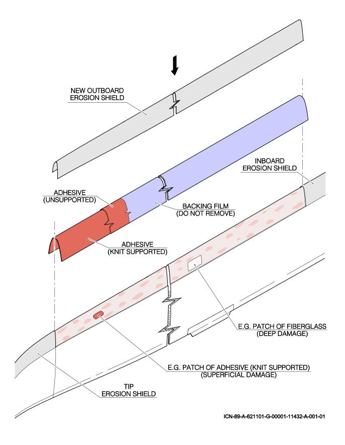
Figure 5 – First adhesive application (Typical) (sheet 1 of 2).
