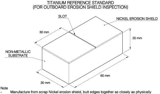
possible and bond onto non-metallic substrate.
