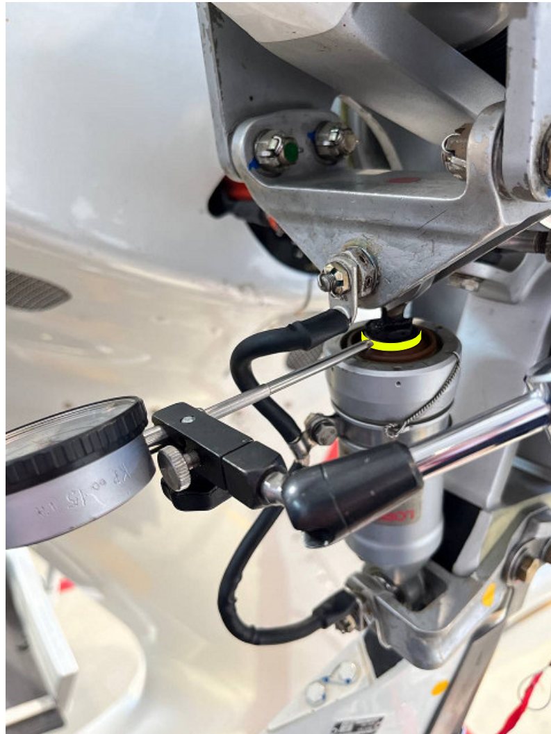
CORRECT POSITION OF THE PLUNGER ON THE SURFACE B
