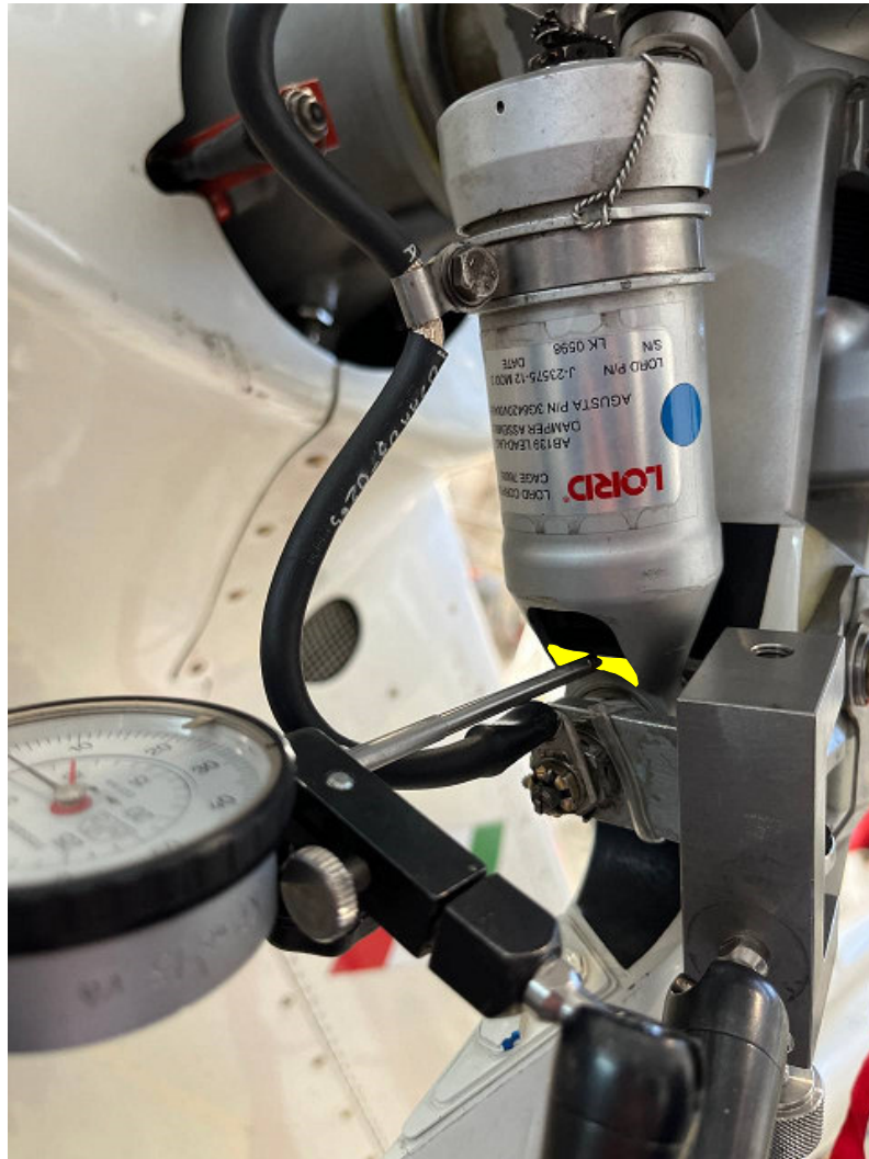
CORRECT POSITION OF THE PLUNGER ON THE SURFACE A
