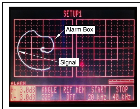
DETAIL B SIGNAL ON ARTIFICIAL DISCONTINUITIES
