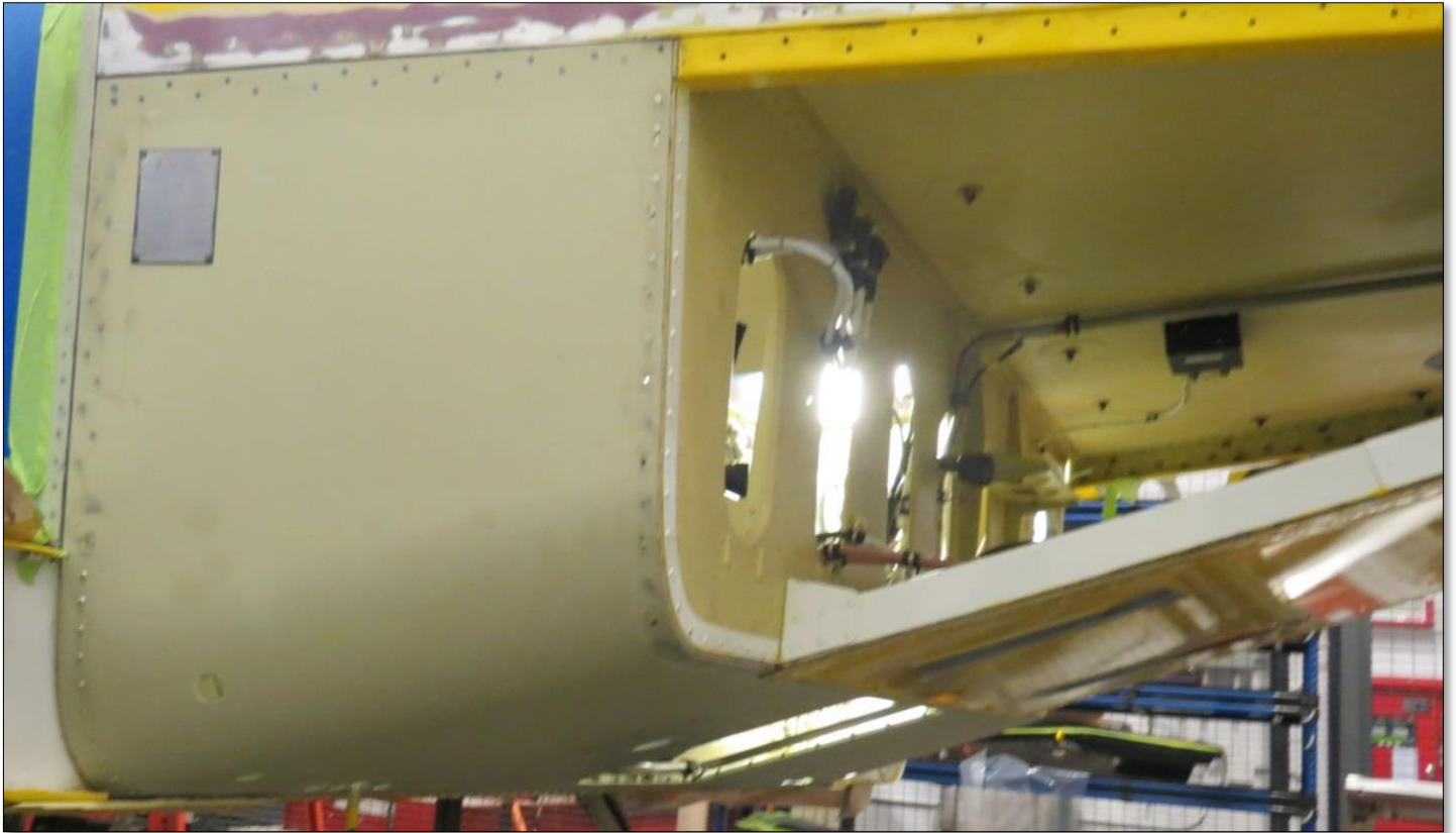
Figure 18 – Forward Lower Panel Assembly Installed (Sheet 1 of 2)
