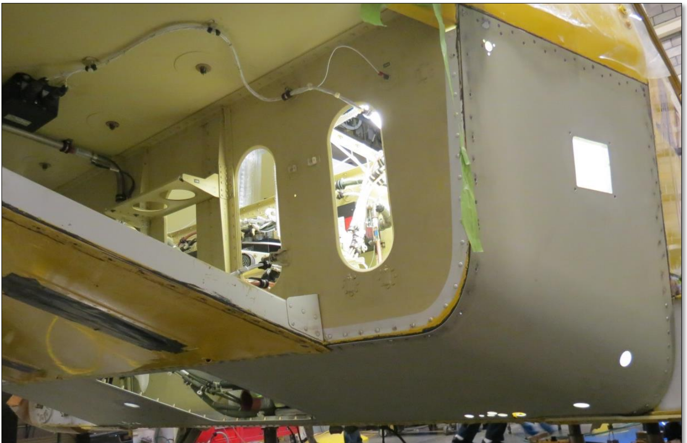
Figure 18 – Forward Lower Panel Assembly Installed (Sheet 2 of 2)
