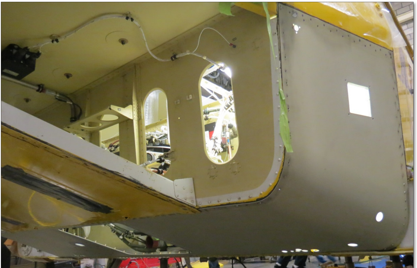
Figure 18 – Forward Lower Panel Assembly Installed ( Sheet 2 of 2 )
