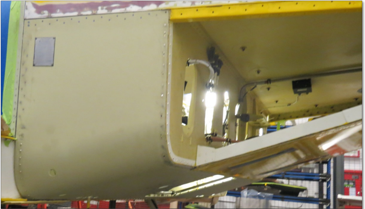
Figure 18 – Forward Lower Panel Assembly Installed ( Sheet 1 of 2 )
