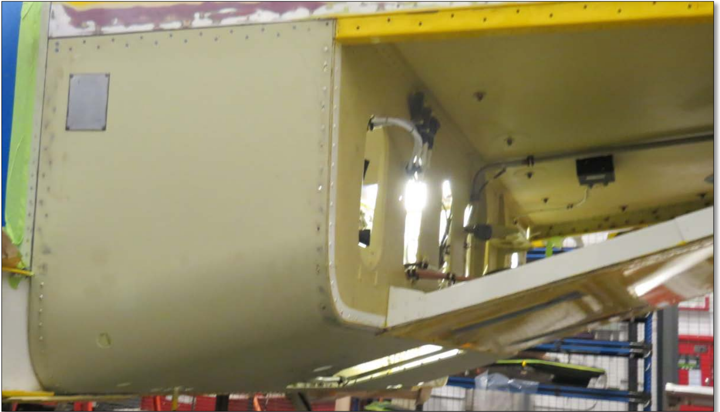
Figure 18 – Forward Lower Panel Assembly Installed (Sheet 1 of 2)
