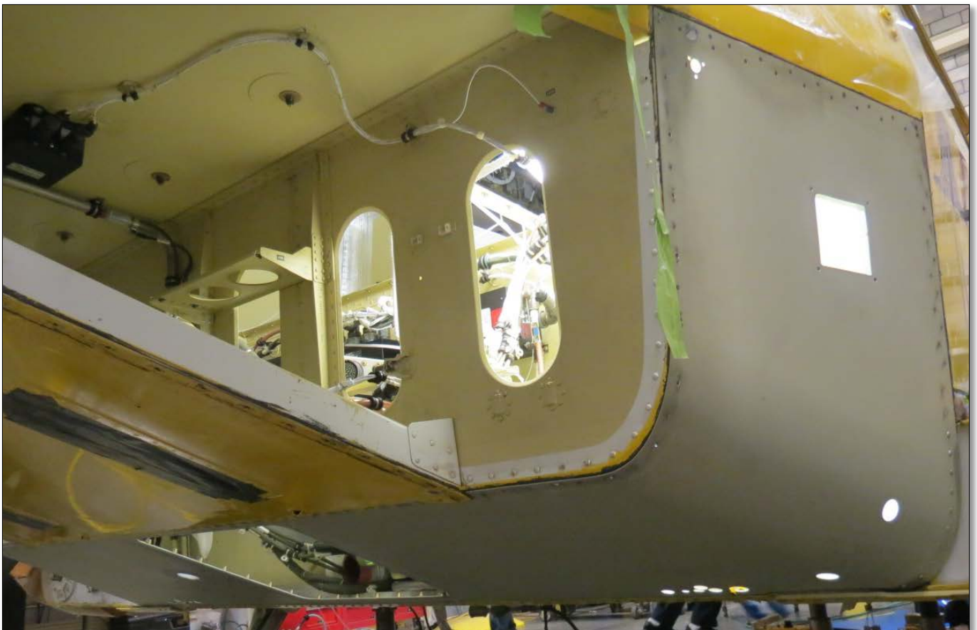
Figure 18 – Forward Lower Panel Assembly Installed (Sheet 2 of 2)
