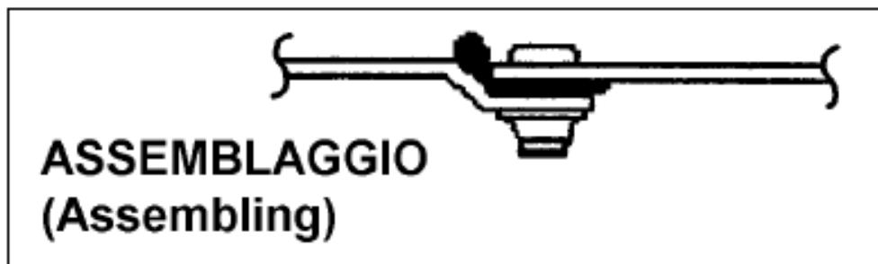
Fig. 6: Check that the squeeze out of sealant is uniform along the edge, visible and enough to allow the correct final finishing of the sealing.
