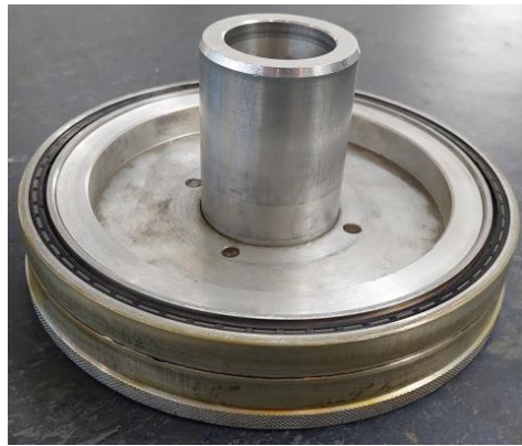
Figure 5 – Duplex bearing ball installed on positioning tool 109-0110-01-109E023A
