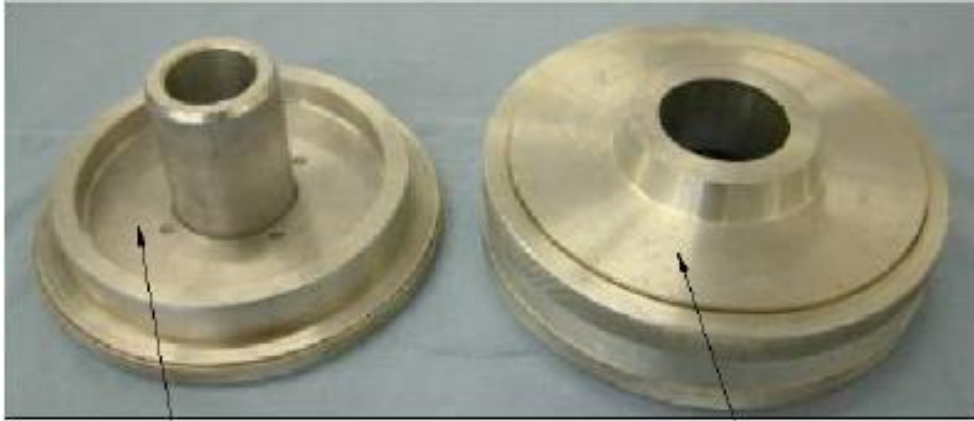
Figure 4 – Positioning tool P/N 109-0110-01-109E023A, “centering support” (to the left) and “base” (to the right)
