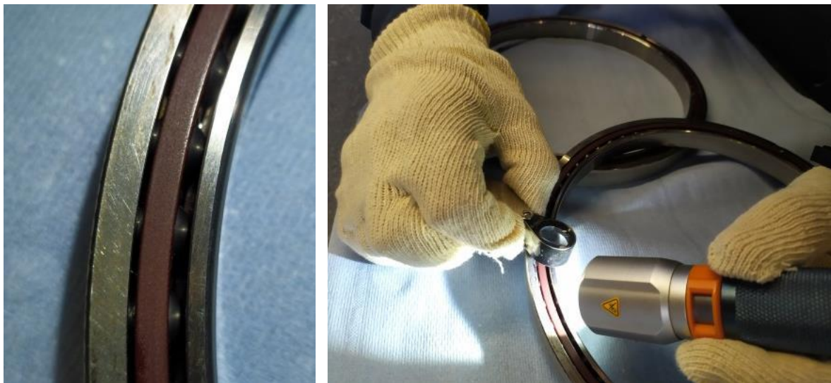
Figure 4 – To the left, detail of the duplex bearing ball; to the right, inspection of inner and outer races.
