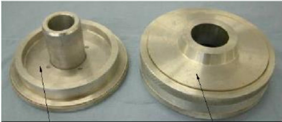
Figure 4 – “Pusher assy P/N 109G6220G03-103” (to the left) and “base assy P/N 109G6220G03-109” (to the right)
