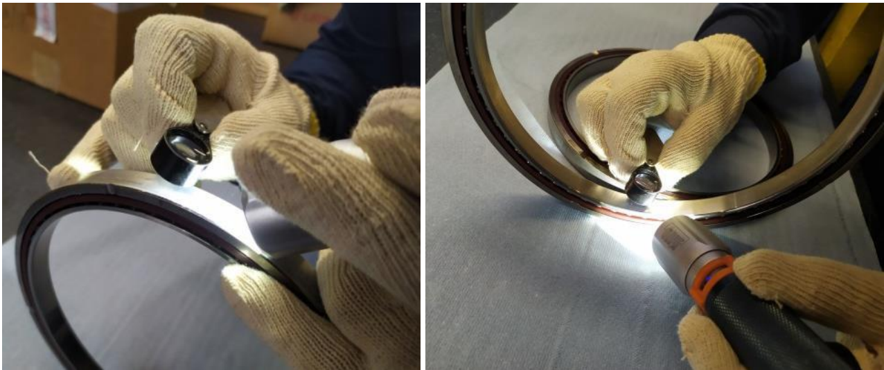
Figure 3 - Outer (to the left) and Inner ring (to the right) inspection of duplex bearing ball.
