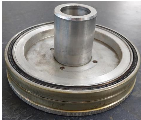
Figure 5 – Duplex bearing ball installed on positioning tool 109G6220G03
