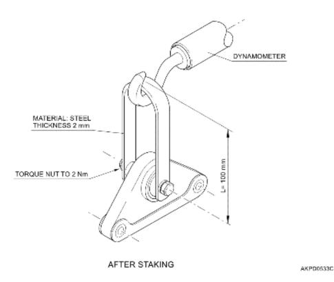
Figure 6 – Spherical Bearing Rotational Torque Check.
