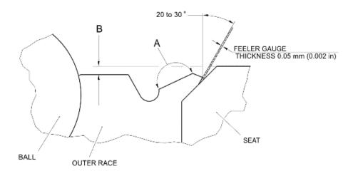
Figure 5 – Spherical Bearing Staked Lip Inspection.
