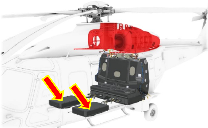
Two Sub Floor Tanks (RH and LH – total capacity 270 l)
