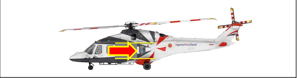
Figure 24 – Sliding Passenger Door - Opening Procedure
