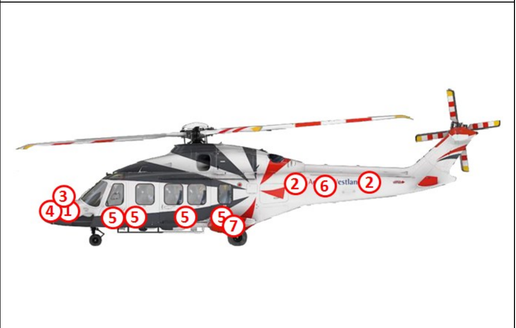
Figure 12 – Hazards – Batteries Location
