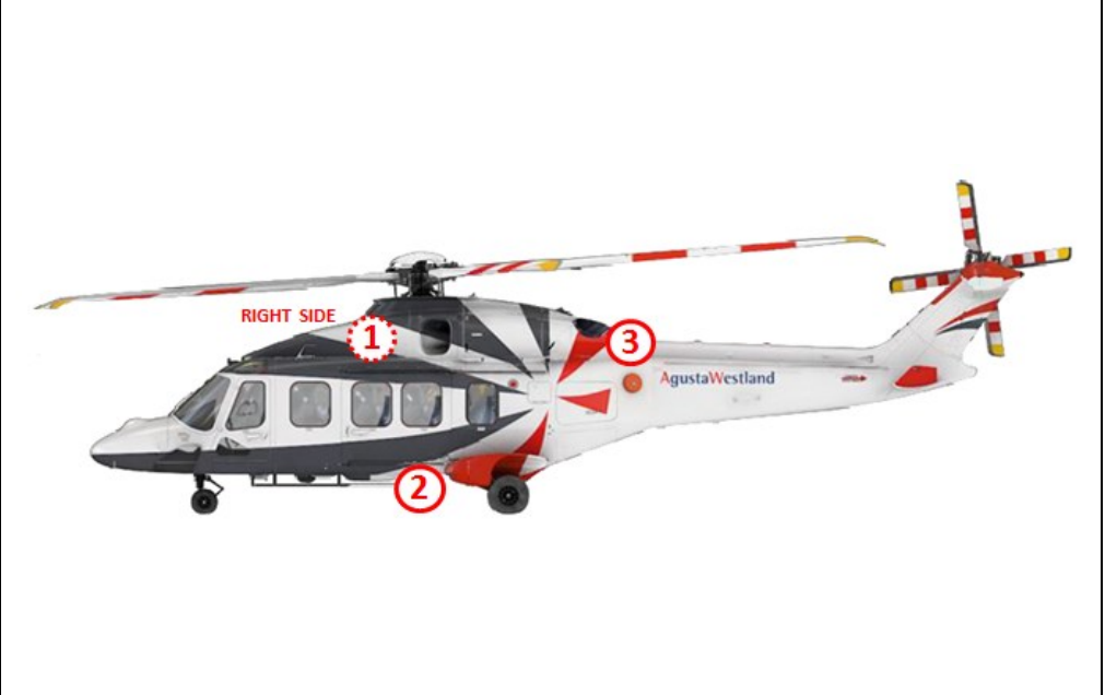
Figure 11 – Hazards – Explosive Charges
