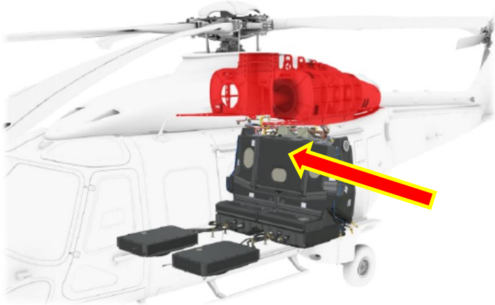
Auxiliary Central Tank (capacity 510 l)
