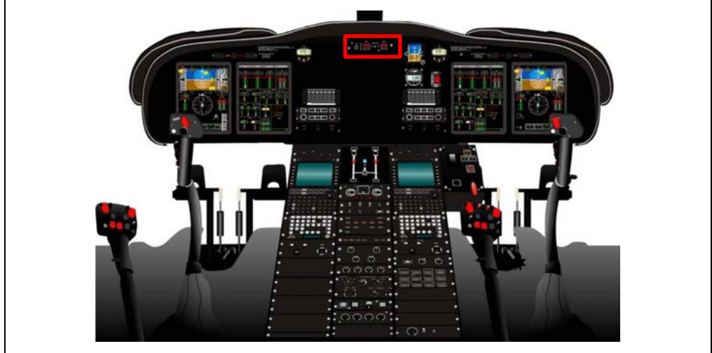
The Engine Fire Detect/Exting. Control Panel is located in the Instrument Panel
