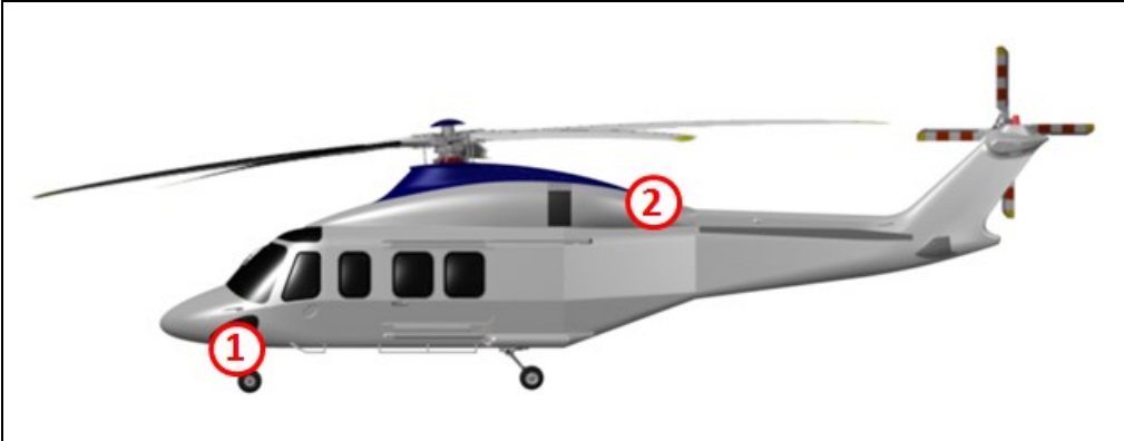
Figure 11 – Hazards – Hot Surfaces
