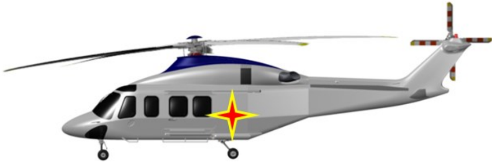
Fuel Tank (capacity 1588 l, see Figure 3)
