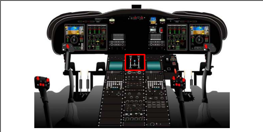
The Fuel Control Panel is located in the Interseat Console
