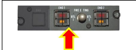
The Engine Fire Detect/Exting. Control Panel is located in the Instrument Panel
