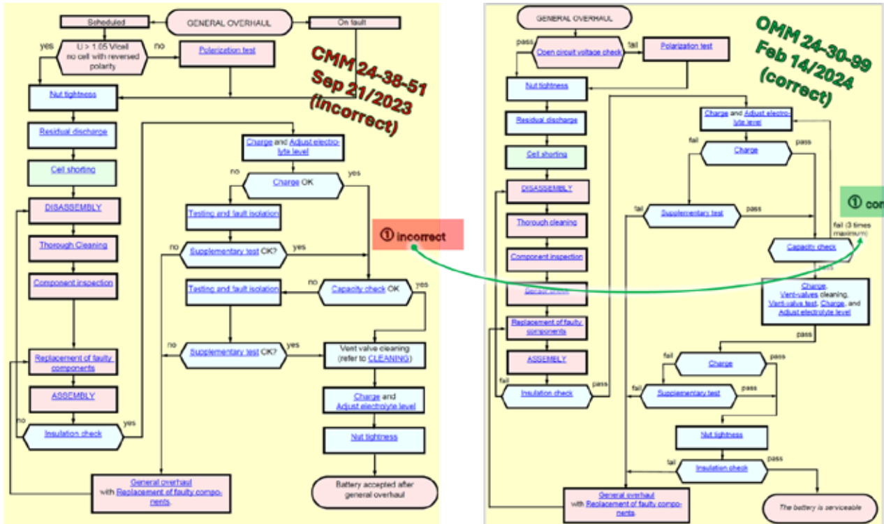
Figure 2 Utilize the Overhaul flow diagram from the Saft OMM 24-30-99 Feb 14/2024 for correction ①
