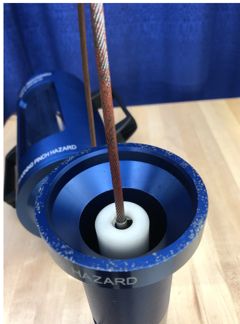
Figure 4. Cable Ball Cover Installation
