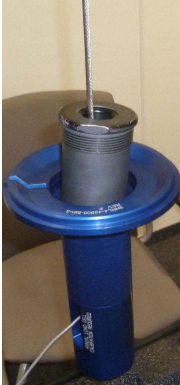
Figure 7. Shock Attenuator Installation (44307-480 hook damper series for hoist 44301-10-7 shown)
