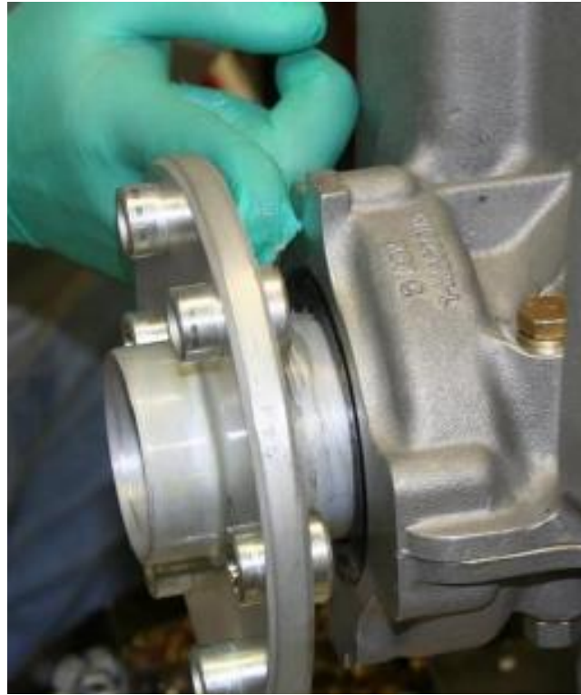
Figure 10 Spread Sealant in Gap Between Case & Seal
