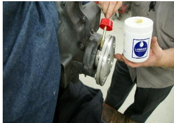
Figure 16 Lubriko M-6 Grease, Engine Oil or Equivalent Applied to the Crankshaft
