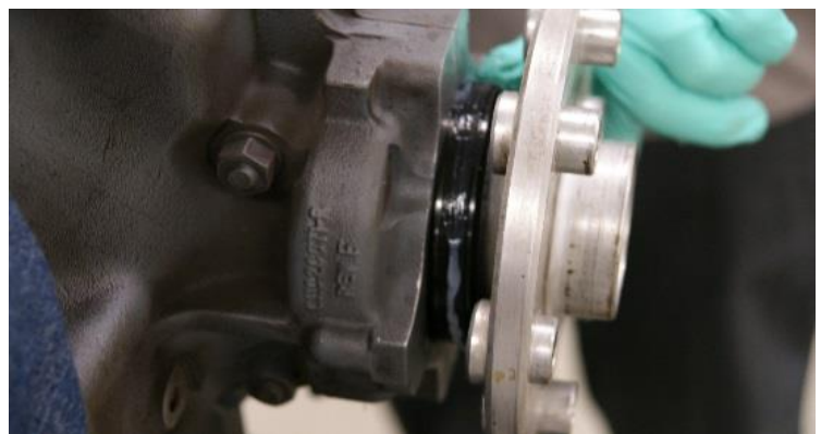
Figure 26 Working the Sealant into the Seal Grooves
