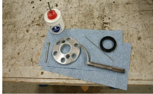
Figure 11 Tools Required for Solid-Ring Crankshaft Oil Seal Installation
