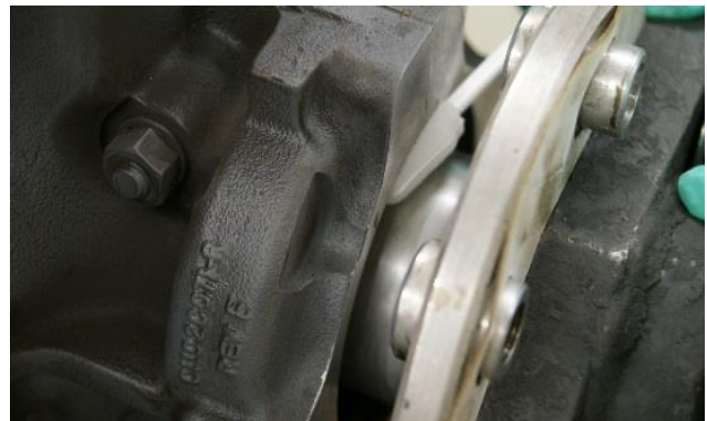
Figure 7 Using a Swab to Clean Away Deposits
