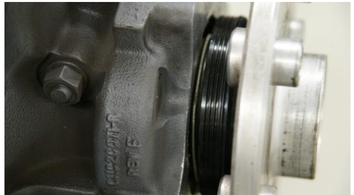
Figure 22 Spring Installed in Relaxed State.
