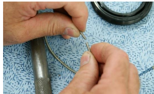
Figure 14 Separating the Spring Threaded Ends
