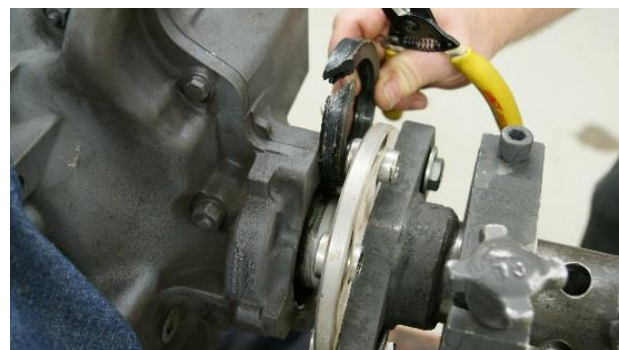
Figure 5 Cutting the Solid-Ring Crankshaft Oil Seal
