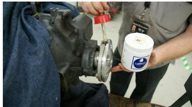
Figure 17 Applied Lubriko M-6 Grease, engine oil or equivalent to the Crankshaft Flange
