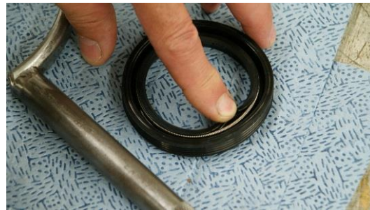
Figure 12 Locating the Internal Spring
