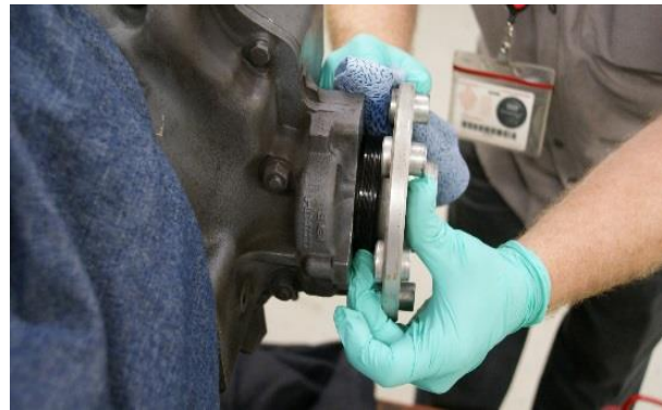
Figure 24 Cleaning the Solid-Ring Crankshaft Oil Seal
