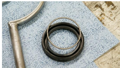
Figure 13 Internal Spring Removed
