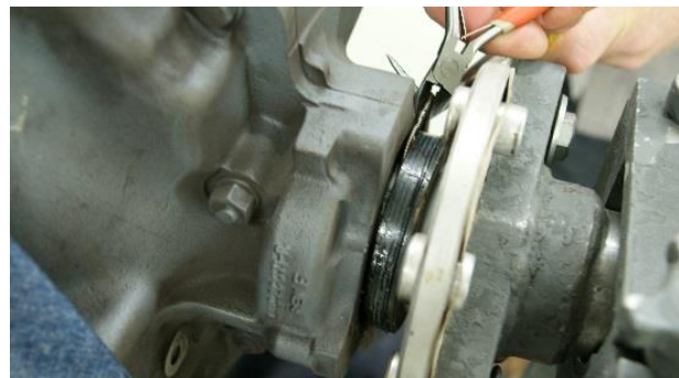
Figure 4 Cutting the Internal Spring
