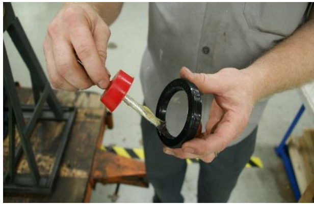
Figure 18 Lubriko M-6 Grease, engine oil or equivalent Applied to the Inside of the Solid-Ring Crankshaft Oil Seal
