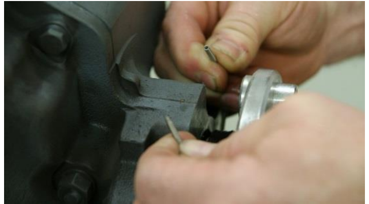
Figure 21 Installing the Spring Behind the Solid-Ring Crankshaft Oil Seal
