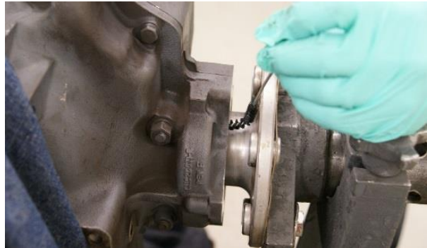
Figure 6 Using Spiral Brush on Hard Deposits
