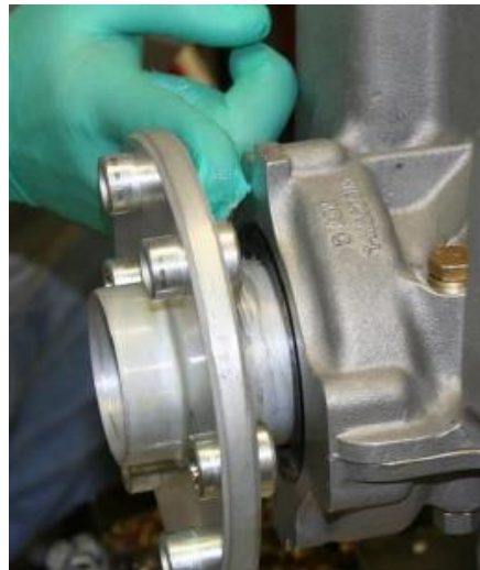
Figure 28 Spread Sealant in Gap Between Case & Seal
