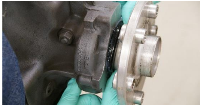
Figure 27 Installing the Solid-Ring Crankshaft Oil Seal into the Crankcase
