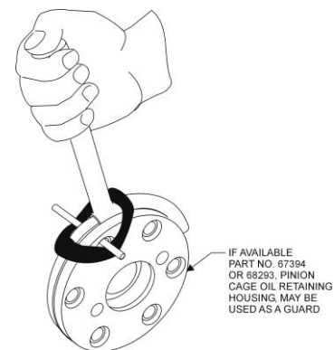
Figure 20B Guard Over the Front of the Flange
