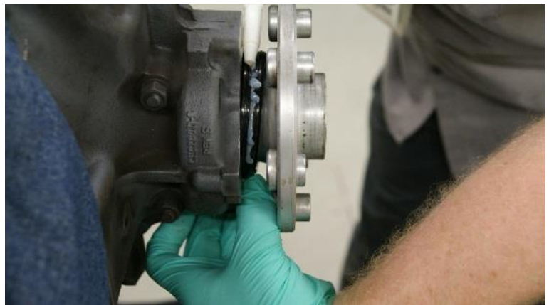
Figure 25 Applying Permatex® Optimum Max Flex Black (P/N 27037)
