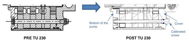
In addition, the cover is changed and then a plug is no more necessary (and this prevents possible seepage).
