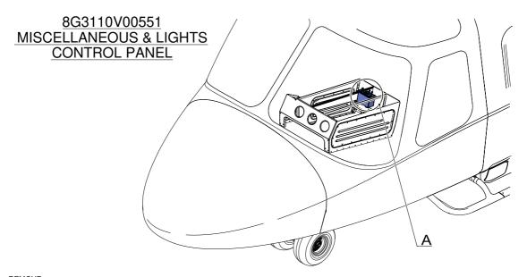
REMOVE: 8G3110V00451 MISCELLANEUS CONTROL PANEL INSTALL: 8G3110V00551 MISCELLANEOUS & LIGHTS CONTROL PANEL
