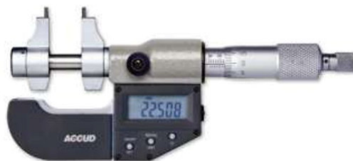
Figure 48: Example of millesimal micrometer for internal dimensions
