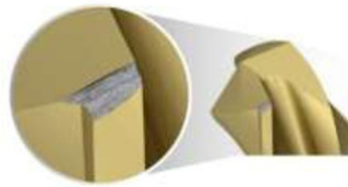
Figure 39: Example of chipping of the main cutting edges
