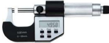
Figure 46: Example of millesimal micrometer for external dimensions
