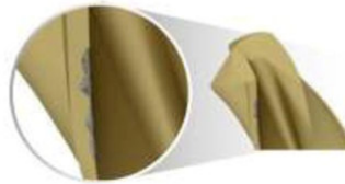
Figure 40: Example of band chipping
