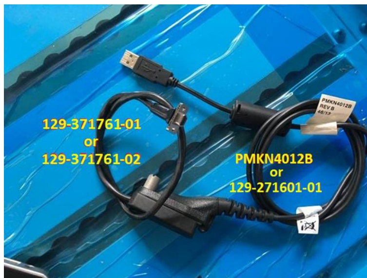
Figure 3-2: Cables used to install APX module(s) configuration file(s)
