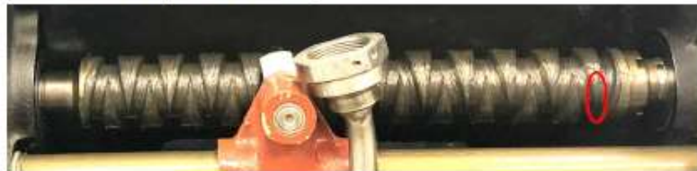
Localization of tips at the intersection of the left and right threads of a winding screw
