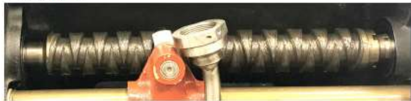
Correct application of grease to the winding screw
