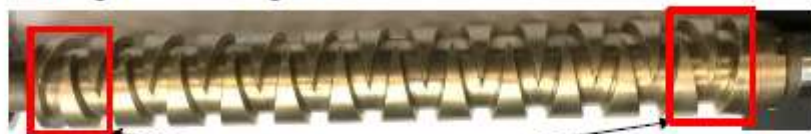
Guiding fork inversion areas (inducing the reversal of direction of displacement of the cable guide)
