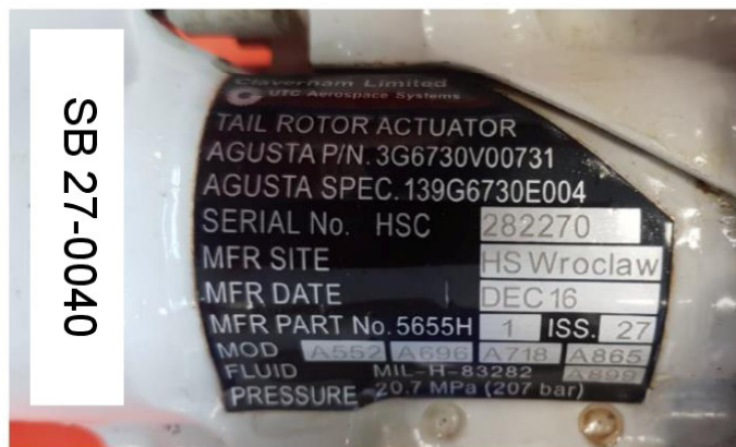
Figure 4: Identification of the SB number on the unit (the shown label is the one of the configuration 5655H1. Reference only)
