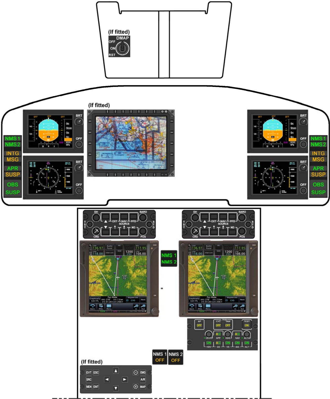
Figure 3: Dual GTN 750H GNSS RNAV system controls and displays
