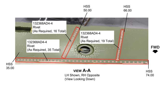
NOTE: Only the areas highlighted in red needs to be inspected for magnetic fasteners.
