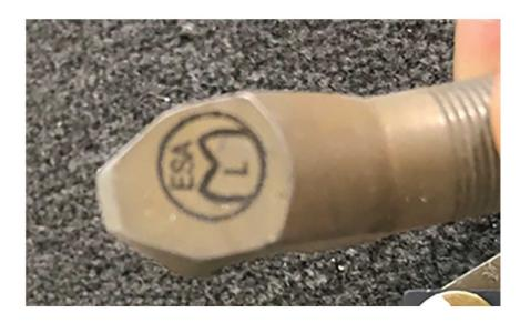
**NOTE:** The inspection mark is on the bottom side of the hook.
