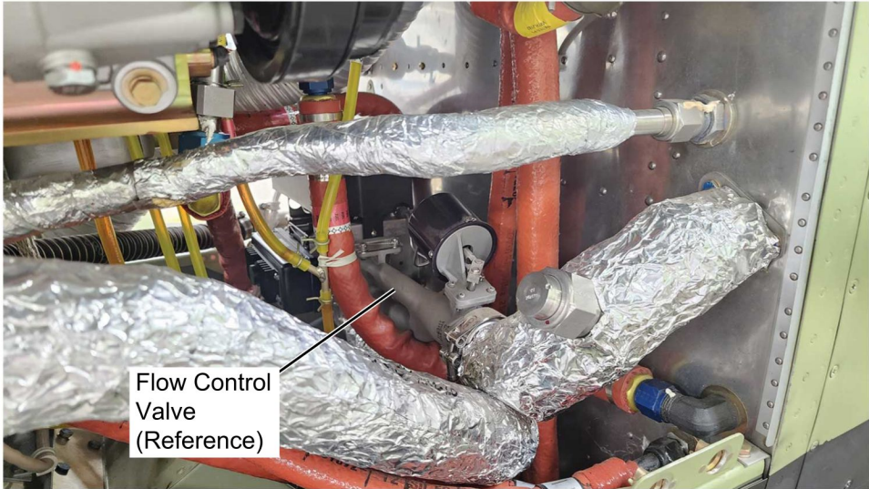
Before Insulation Installation View Looking Outboard at Left Engine (Model 200GT Shown)
