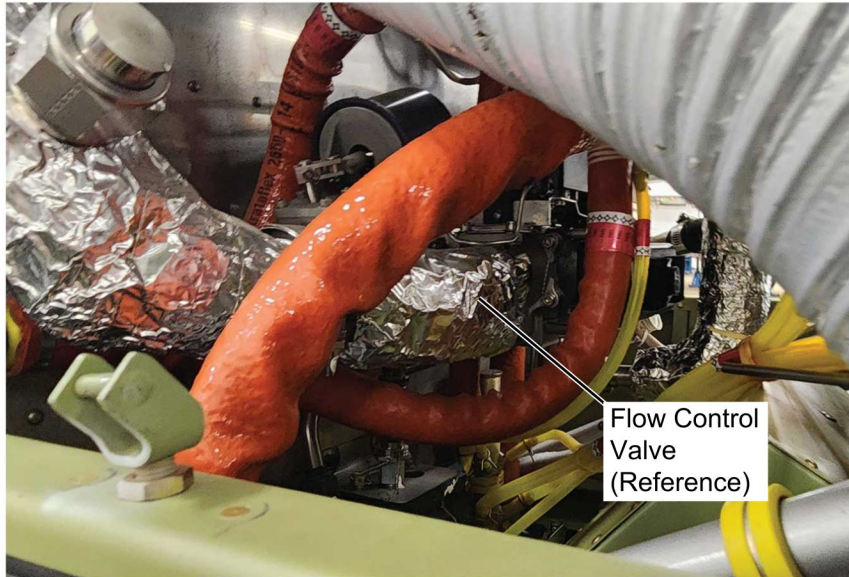
After Insulation Installation View Looking Outboard at Left Engine (Model 200CGT Shown)
