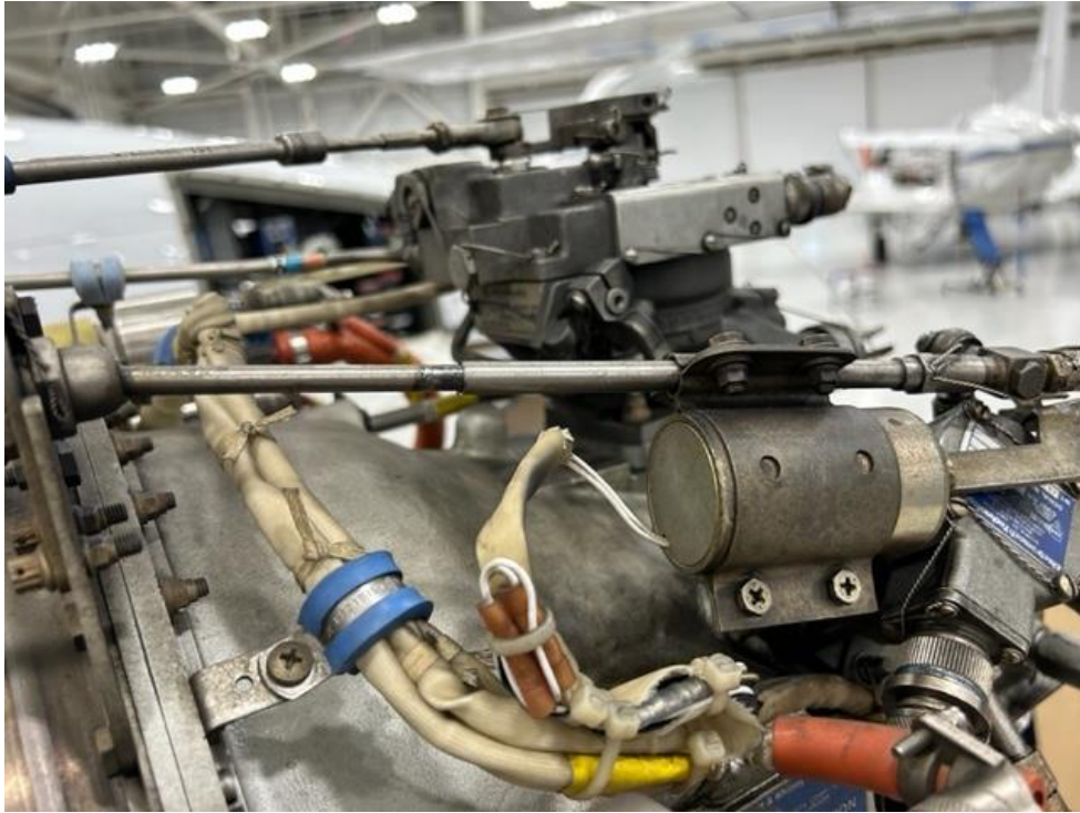
Ground Idle Solenoid without support or RTV
