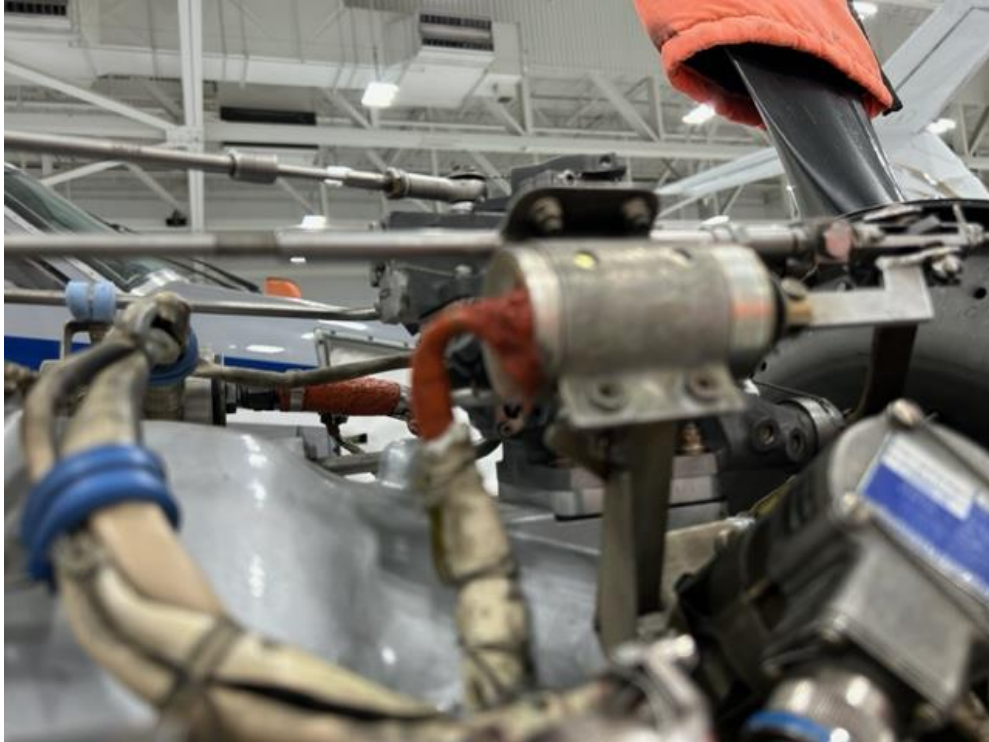
Ground Idle Solenoid with support and RTV
