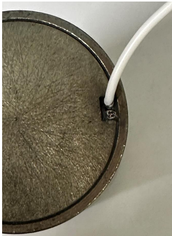
Ground Idle Solenoid with a Broken Wire
