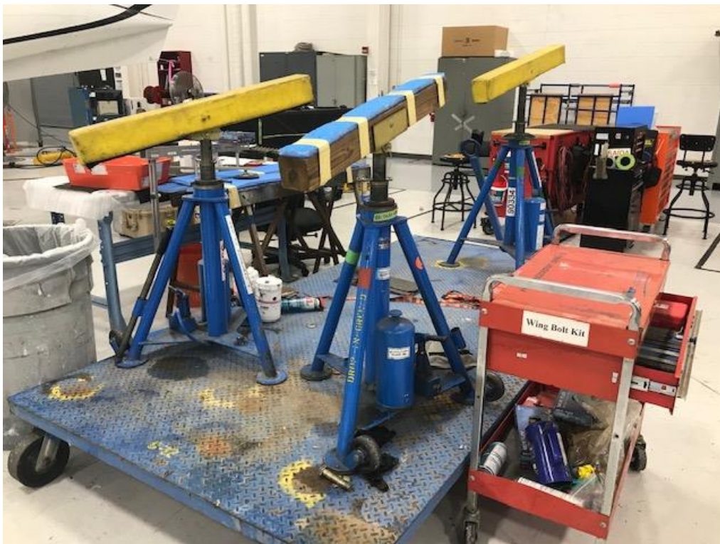
Modified Jacks to Support the Wing
