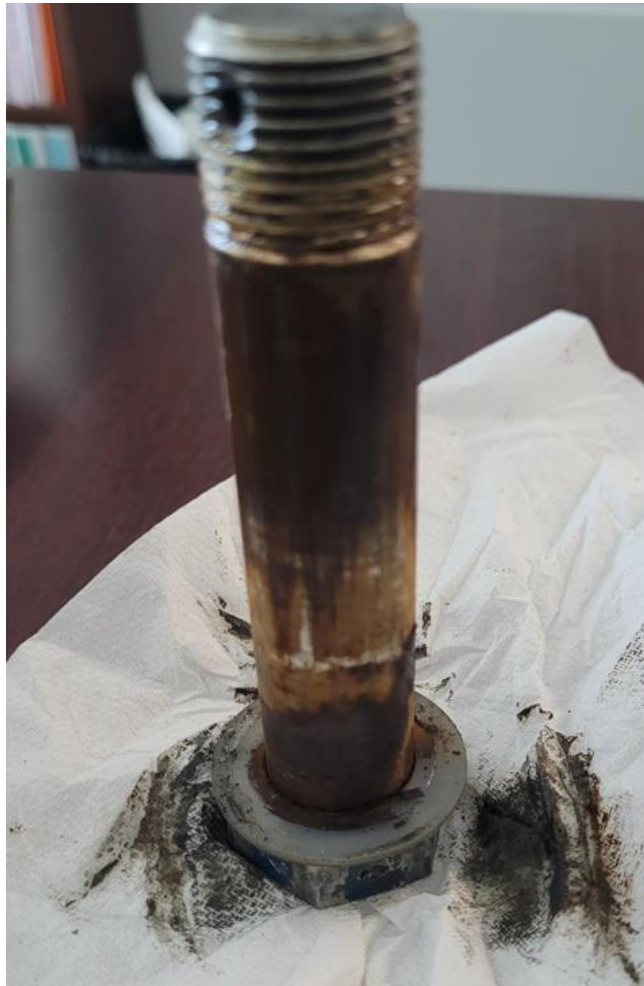
Corroded Wing Bolt
