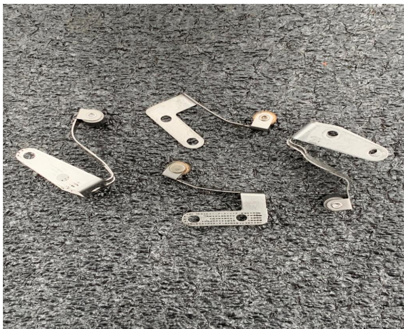
Damaged Switch Actuators
