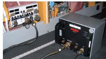
Fixed Installation Kit Example (On ARRIUS 2B1 - 2B1A - 2B2)
