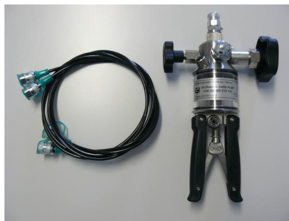
Hand pump and miniflex for gauge checking
