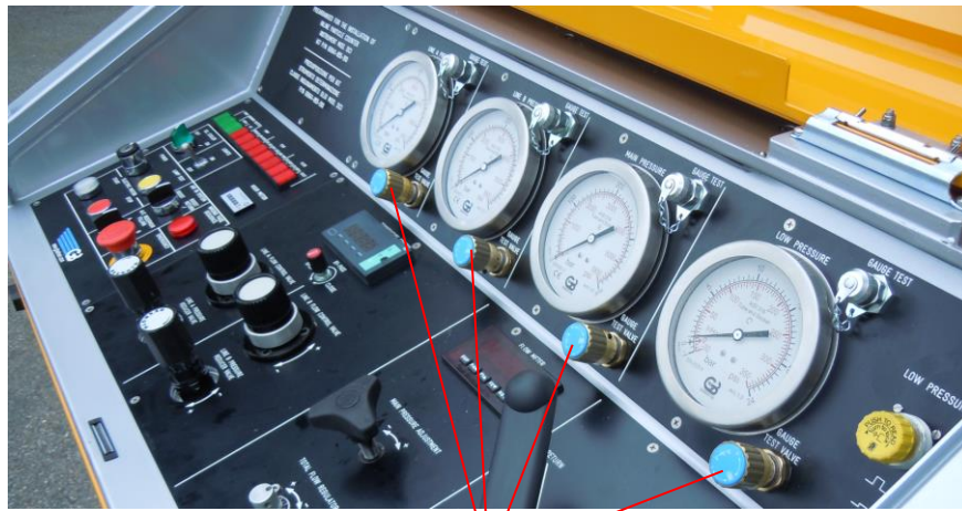
“GAUGE TEST VALVE”
