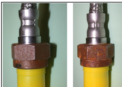
Figure 2: Picture showing obvious surface corrosion.
