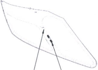
LOCATION OF INTERIOR PLACARD ON AFT CO-PILOT DOOR
