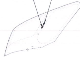
LOCATION OF INTERIOR PLACARD ON AFT PILOT DOOR
