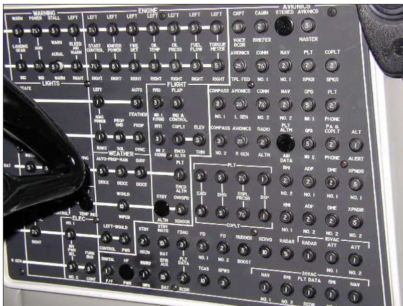
Figure C- 7: Co-pilot's Circuit Breaker Panel
