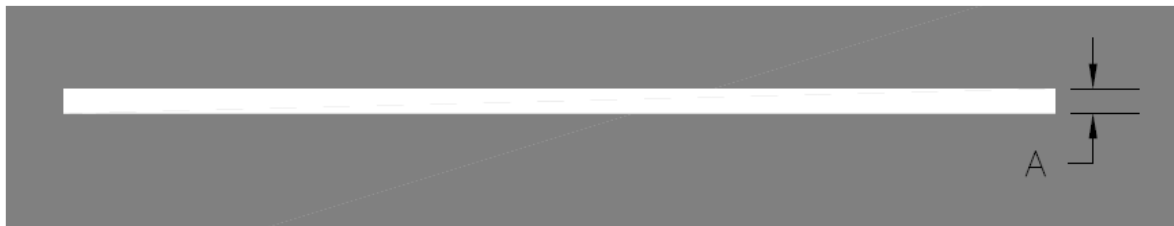
Figure 15-2. Equipment parking marking
