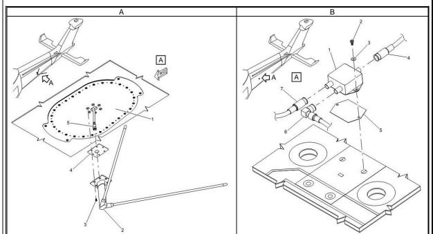
49 -1 APU Inlet Barrier Filter Actuator
