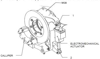
Secure the calliper in the down position connecting the bolt holes (1) and (2) with a tie-wrap strap. Secure the free connector of the actuator using a tie-wrap strap. Pull the PWR and the CONTR circuit breakers on the RTR BRK section of the overhead circuit breaker panel. Secure the system by locking all the deactivated circuit breakers and tag accordingly.
