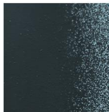
Not acceptable: P20 primer partly covered
