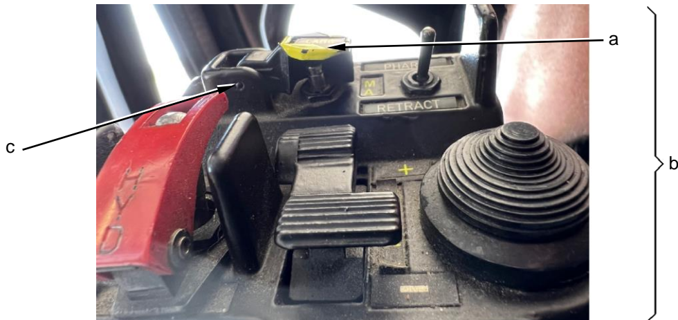
Figure 9 - Position of the safety-cap and pin
