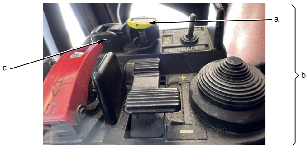
Figure 9 - Position of the safety-cap and pin
