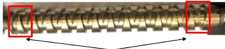
Guiding fork inversion areas (inducing the reversal of direction of displacement of the cable guide)
