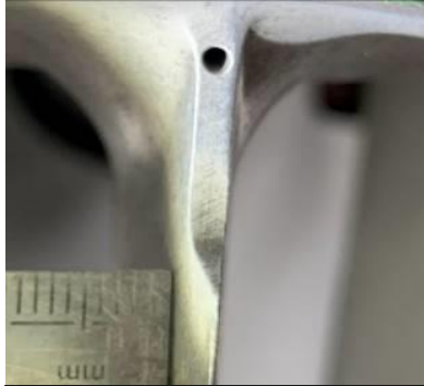
Incorrect ruler location: NOK
