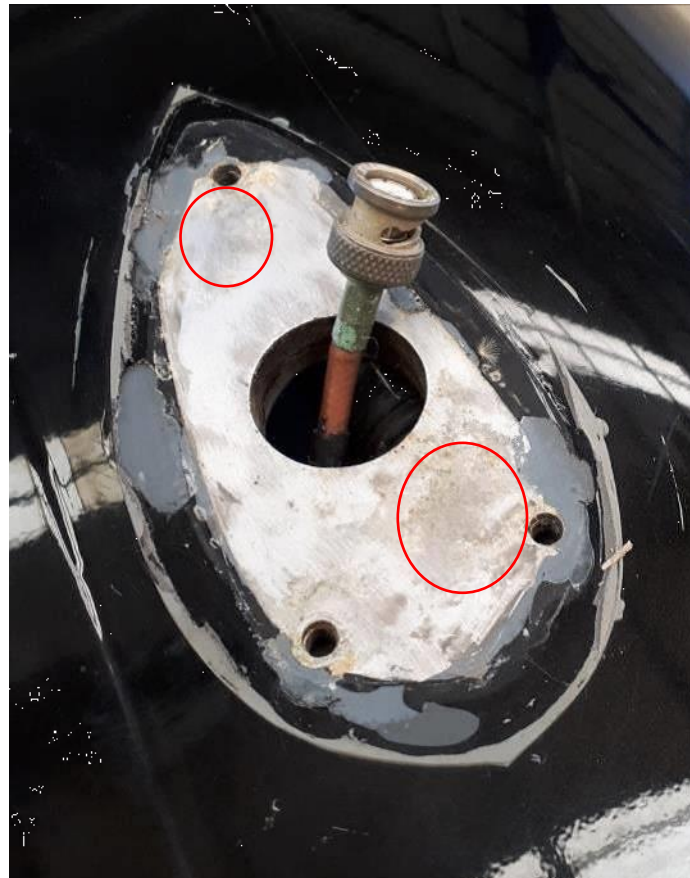
Example of corrosion and aluminium oxide
