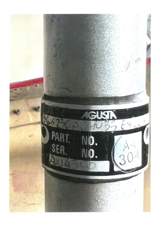
DRANGE - UPPER ROD END ASSY P/N: 3G6230A01133 : S/N: MCR 08970
