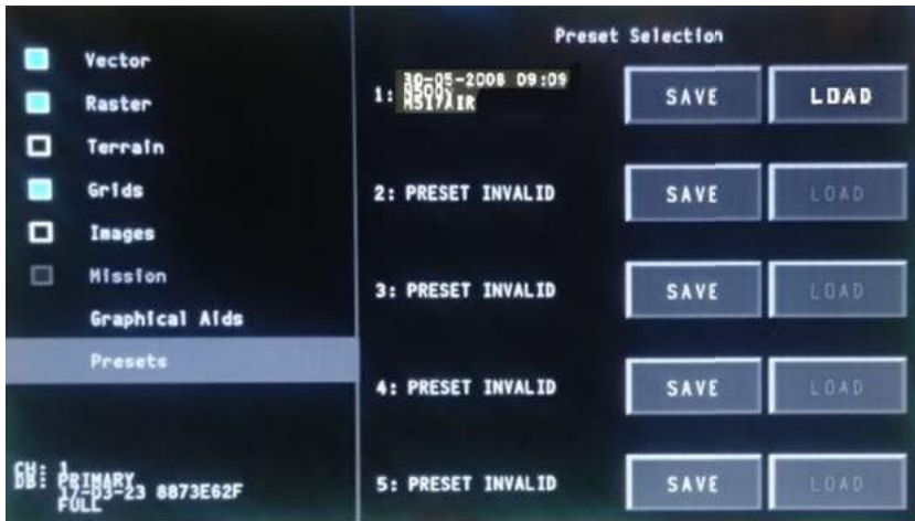
Figure 5-50 PRESETS type management by MFD (2 of 2)
