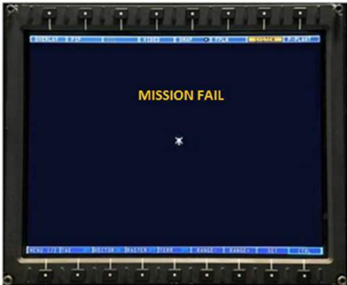
Figure 8-1 “MISSION FAIL” message on MFD
