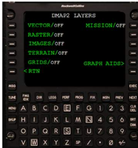
Figure 5-11 Setting Displayed Map Types by MCDU
