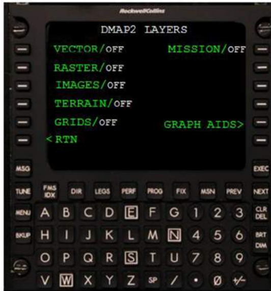
Figure 5-48 Mission vector activation/deactivation by MCDU
