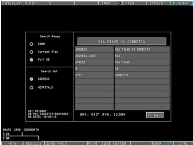
Figure 5-51 SEARCH function management by MFD (4 of 4)
