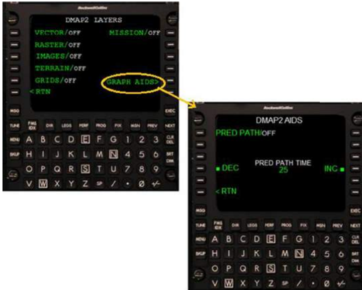
Figure 5-31 PREDICTED INTERVAL Time definition by MCDU
