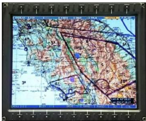
Figure 5-45 TERRAIN DATA TRANSPARENCY change by MFD (3 of 3)
