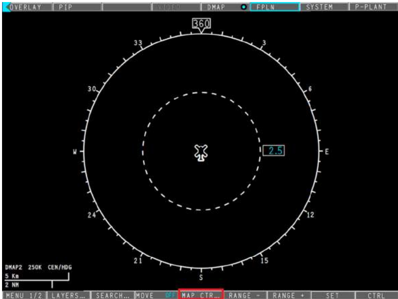
Figure 5-20 Map Center Modes on Main Control Menu
