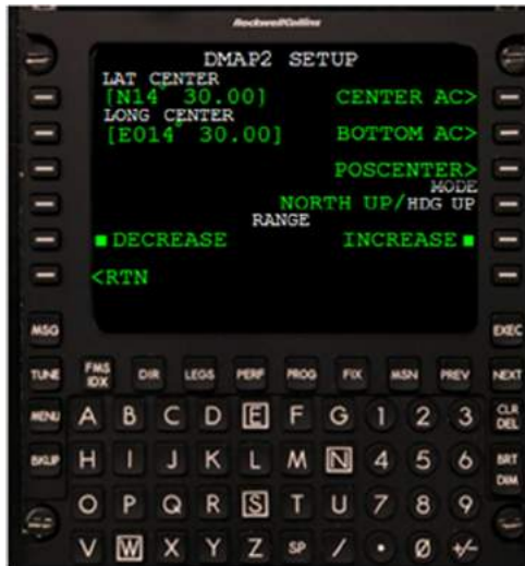
Figure 5-3 Map Orientation Mode by MCDU
