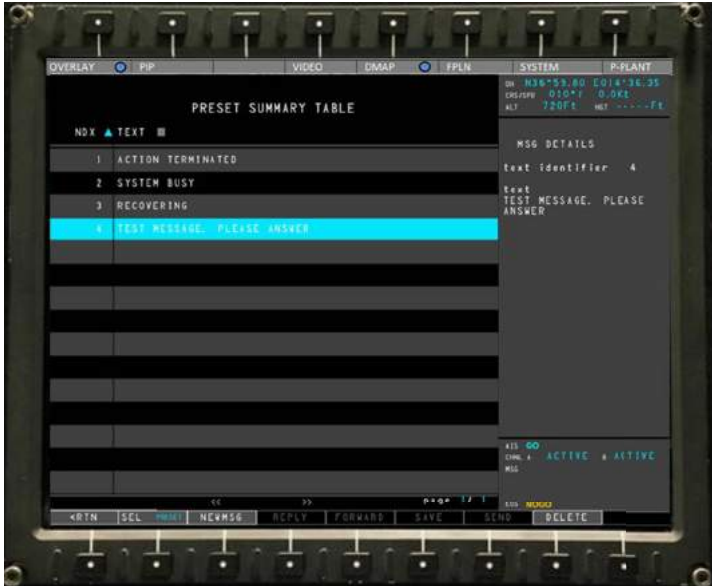
Figure 6-13 Forward, reply and delete an AIS Message by MFD control menu (5 of 5)
