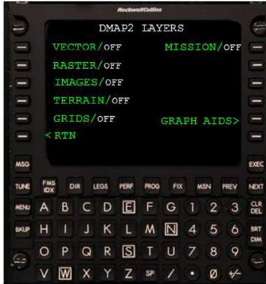
Figure 5-38 TERRAIN DATA presentations by MCDU
