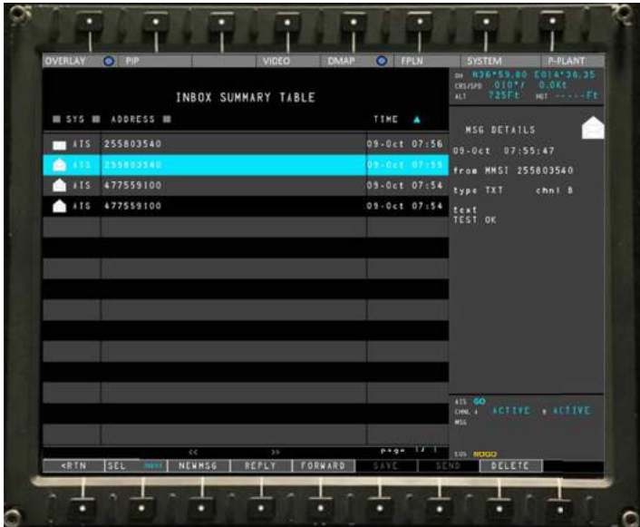
Figure 6-13 Forward, reply and delete an AIS Message by MFD control menu (3 of 5)
