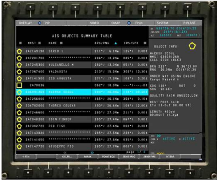
Figure 6-5 AIS Objects Summary Tables (example) (1 of 2)
