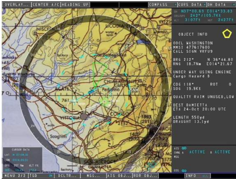
Figure 6-19 EOS LOS and FOV display
