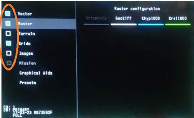
Figure 5-10 DMAP control functions on the MFD DMAP LAYERS CONTROL PANEL
