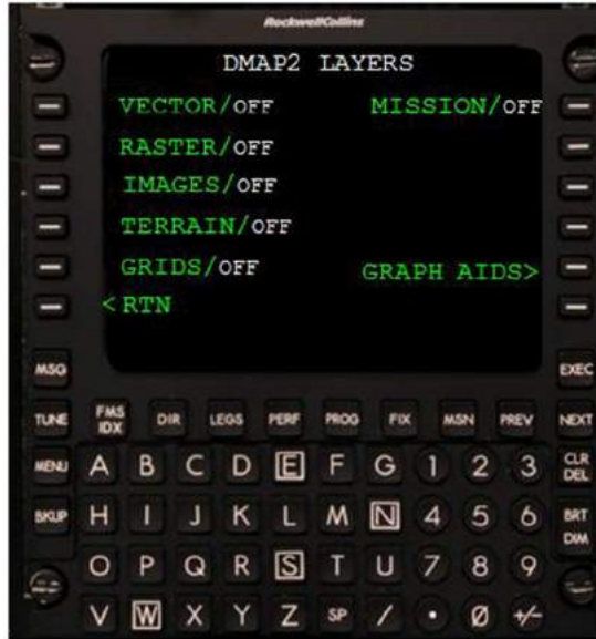
Figure 5-28 Grids activation/deactivation by MCDU
