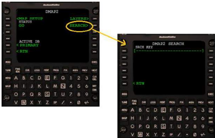
Figure 5-52 SEARCH function management by MCDU (1 of 2)
