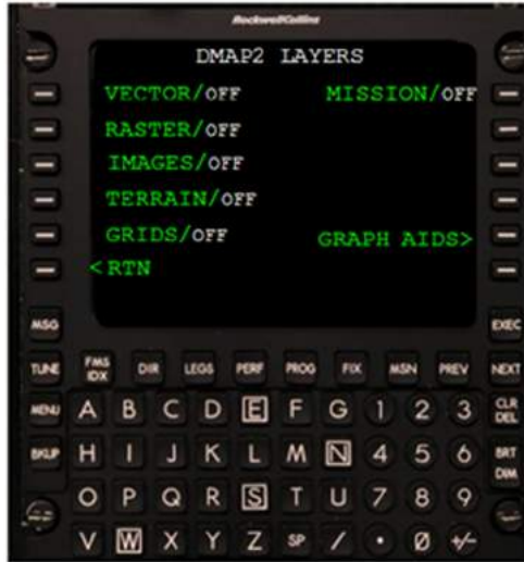
Figure 5-17 Images activation/deactivation by MCDU
