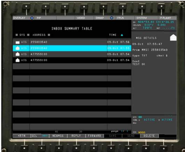
Figure 6-12 AIS INBOX Summary Table (example)
