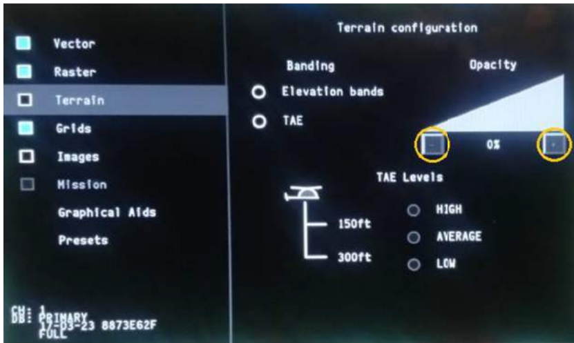
Figure 5-40 TERRAIN DATA TRANSPARENCY change by MFD (1 of 3)
