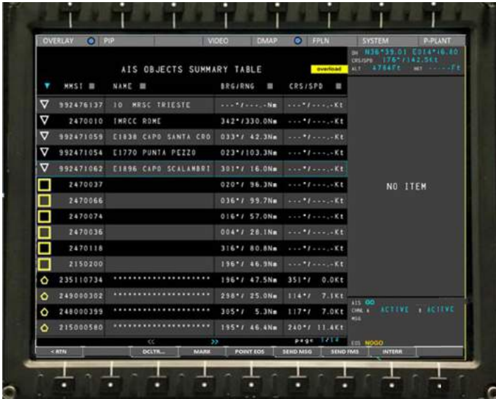
Figure 6-5 AIS Objects Summary Tables (example) (2 of 2)
