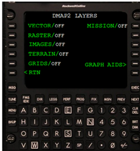
Figure 5-11 Setting Displayed Map Types by MCDU
