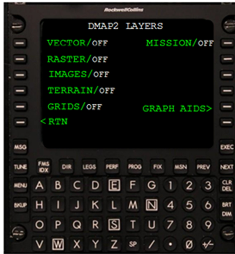
Figure 5-17 Images activation/deactivation by MCDU
