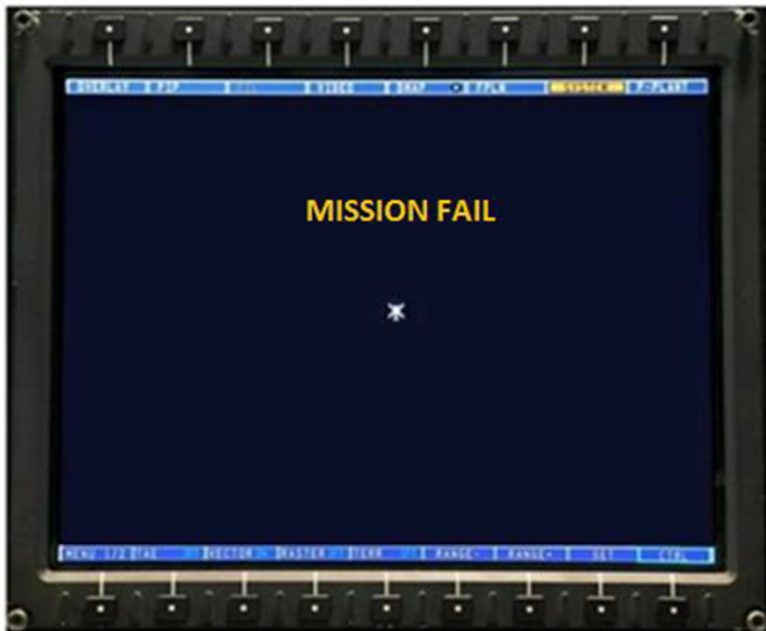
Figure 8-1 “MISSION FAIL” message on MFD
