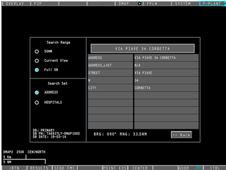
Figure 5-51 SEARCH function management by MFD (4 of 4)
