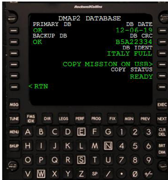
Figure 5-46 MISSION VECTORS copy from DTD to USB by MCDU
