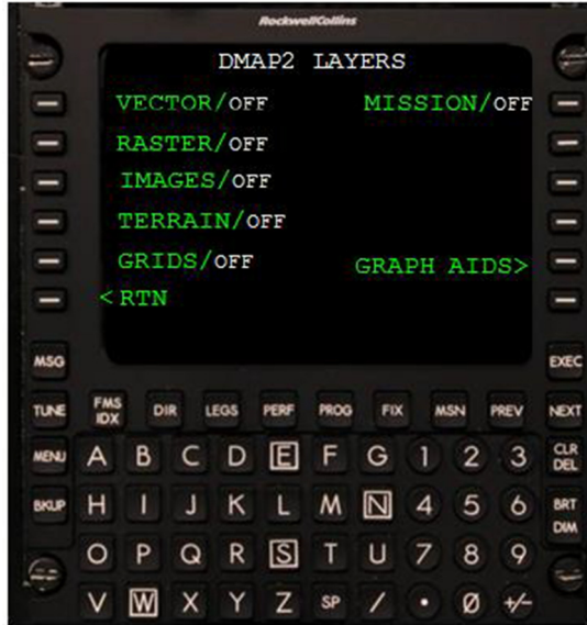
Figure 5-38 TERRAIN DATA presentations by MCDU
