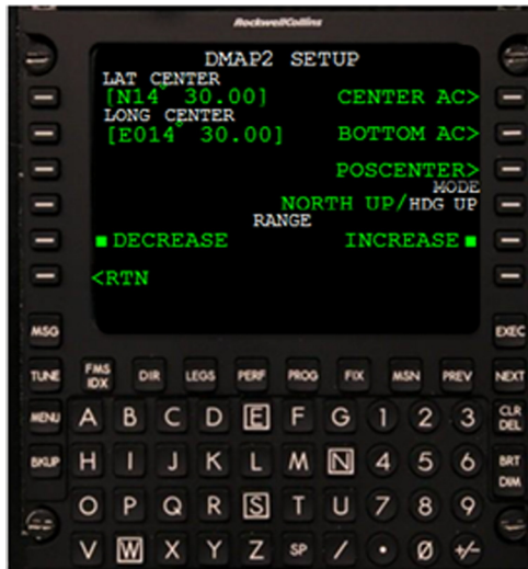
Figure 5-3 Map Orientation Mode by MCDU
