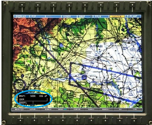
Figure 5-15 Range indication for displayed map on MFD
