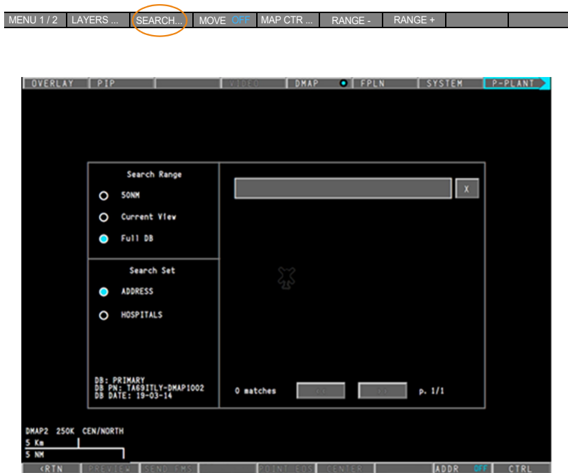
Figure 5-51 SEARCH function management by MFD (1 of 4)
