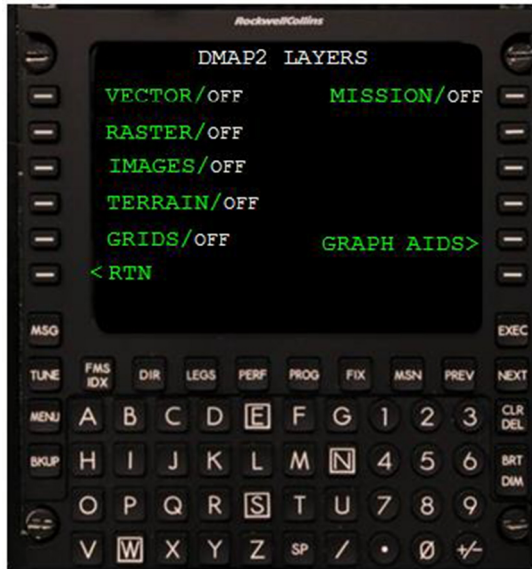
Figure 5-48 Mission vector activation/deactivation by MCDU
