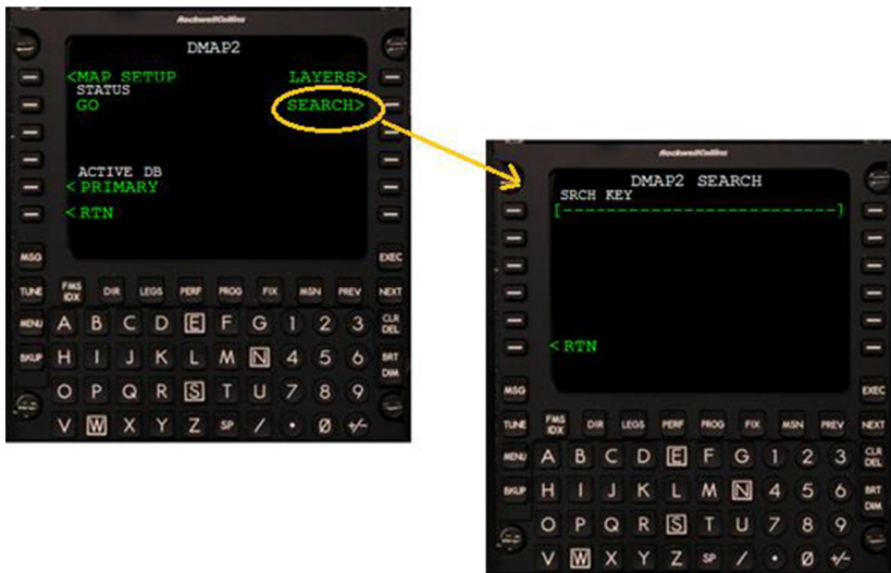
Figure 5-52 SEARCH function management by MCDU (1 of 2)
